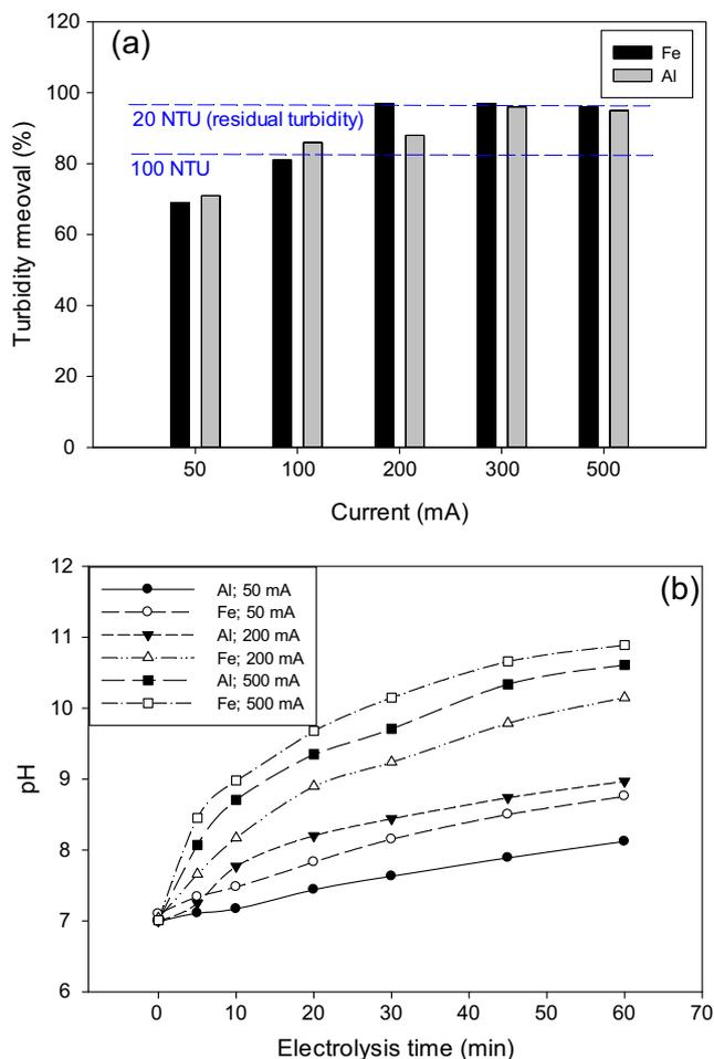
**Fig. 4** **a** Turbidity removal. **b** pH evolution for Fe and Al electrodes. Note that the *dashed lines* in panel (**a**) represent residual turbidity (NTU). Operating conditions: temperature, 20 °C; volume, 0.5 L; supporting electrolyte, 42 mmol L<sup>-1</sup> of NaCl; pH<sub>0</sub>=7.0; 300 rpm; electrolysis time, 60 min
