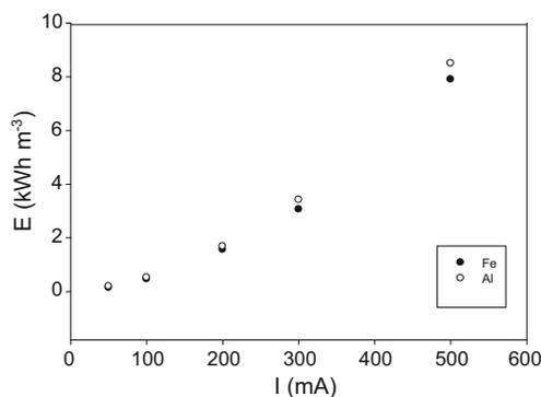
**Fig. 7** Electrical energy consumption in EC of Se(0) with Al or Fe electrodes
