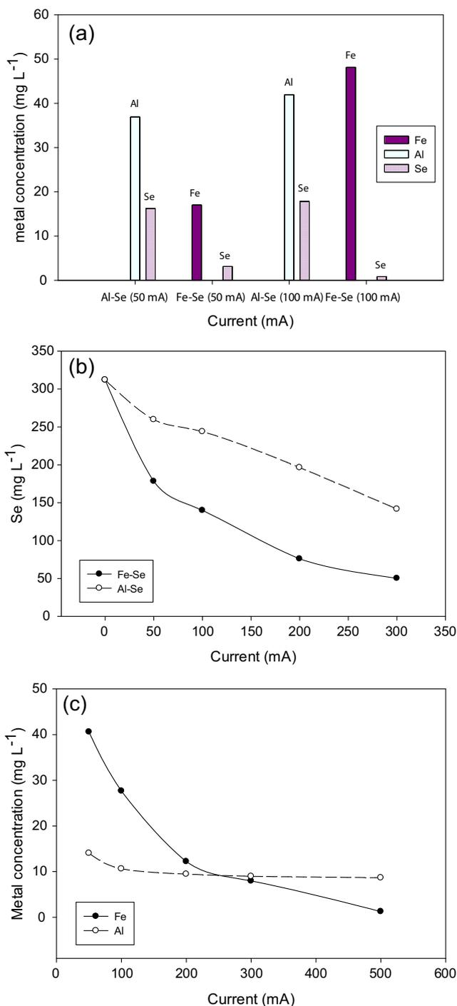
**Fig. 5** a TCLP of Se-Al and Se-Fe sediments, b residual Se in the supernatant of Al and Fe electrode experiments. Note that “0 mA” corresponds to the initial Se content of the suspension before EC treatment, and c residual Al and Fe from the supernatant of Al and Fe electrode experiments. Note that “0 mA” corresponds to the initial Se content of the suspension before EC treatment
