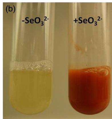
**Fig. 2** a Colloidal stability of biogenic red Se(0) produced by *P. fluorescens*. Evolution of the ratio  $C/C_0$  in function of treatment time with  $C_0$  and  $C$  the turbidity (in NTU) at the initial and a giving time, respectively, and **b** biogenic red Se(0) produced by *P. fluorescens* and the control sample (KB medium)
