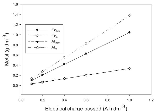
**Fig. 3** Variation of theoretical and measured Al and Fe with the electrical charge passed during EC. Operating conditions: temperature, 20 °C; volume, 0.5 L; supporting media, 42 mmol L<sup>-1</sup> of NaCl; pH<sub>0</sub>=7.0; 300 rpm; electrolysis time, 60 min. Fe<sub>theo</sub> and Al<sub>theo</sub> refer to the theoretical metal dissolved according to Faraday's law (Eq. (6)). Fe<sub>m</sub> and Al<sub>m</sub> are the measured values with charge passed
