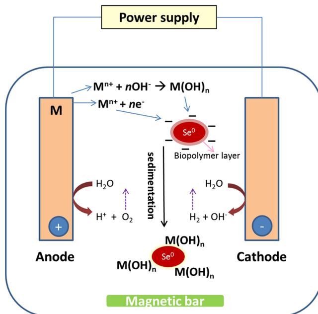
**Fig. 1** Schematic diagram of the electrocoagulation setup. *M*=metal (e.g. Al, Fe), *n*<sup>+</sup>=oxidation state; *M(OH)<sub>n</sub>*=metal hydroxides
