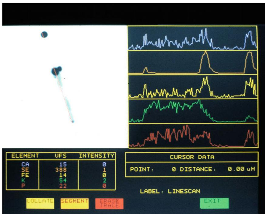
**Fig. 5** Se<sup>0</sup> produced by *Wolinella succinogenes* growing in media containing 0.1 mM selenite. The presence of Ca, Se, Fe, K, and P along the red line indicated in the figure is complemented with the analysis by energy-dispersive X-ray spectrometry provided in the right-hand panel (Barton et al. 2014, used with permission)
